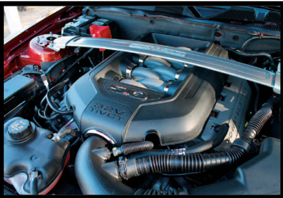
The test drive Mustang featured a 5.0-liter V-8 engine capable of 420 hp.
